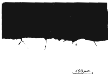
FIG. 3 Character of intergranular corrosion of E1617 alloy in 15% \text{NaNO}_3 . Magnification 200 \times , nonetched
